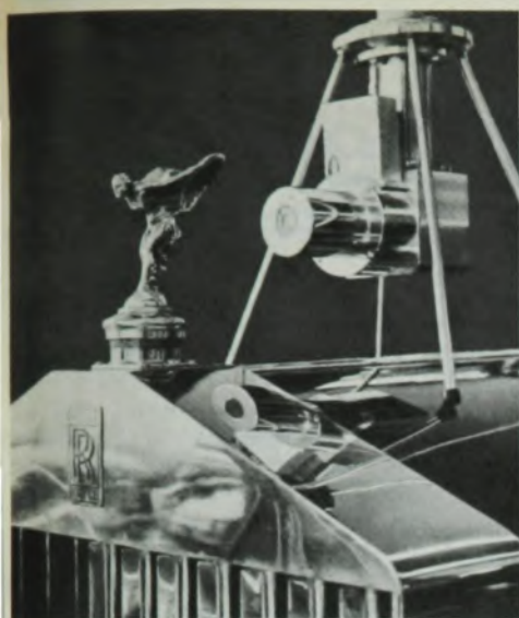
Analysis of hood ornament with KEVEX-RAY spectrometer
