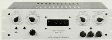
Features: negative high voltage variable to 2000 volts resolution of PMT currents down to 1 picoampere digital accuracy with analog output dark current cancellation recorder drive
