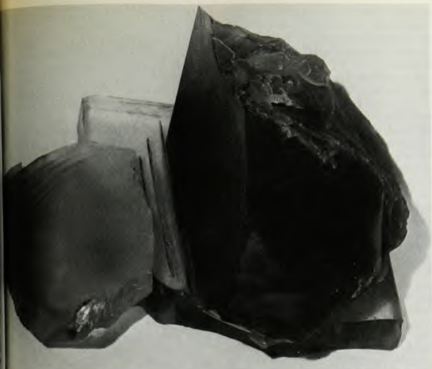
Ultrasonic transducer material. Crystalline quartz in the beginning stages of preparation for use in the development of ultrasonic delay lines. Photo by Bell Laboratories.
