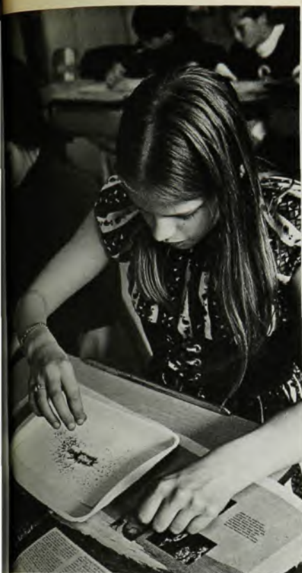
Magnetic field. This girl is sprinkling iron filings on a cardboard tray that conceals a small ferrite magnet. When her pattern is completed to her satisfaction, she will spray it with a transparent glue to fix it semipermanently for classroom display and comparison with the patterns produced by her classmates.
