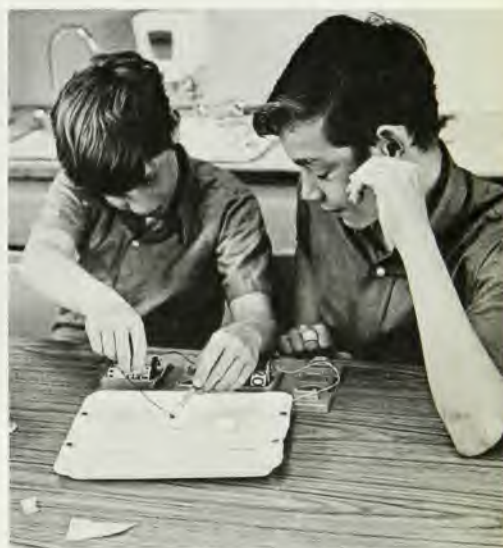
Nichrome wire gets warm when connected to a battery and can melt rubber or char small pieces of paper. These boys are investigating how the length of nichrome wire in the circuit affects its ability to transfer energy.
