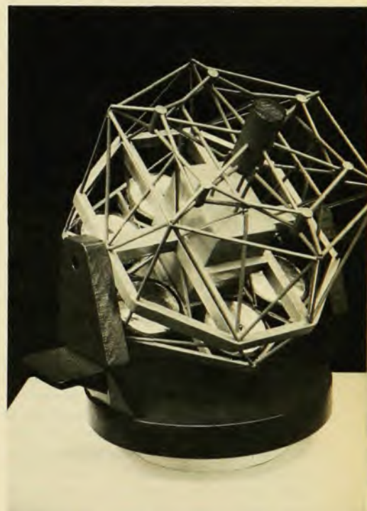
Model of multimirror telescope to be built by University of Arizona and Smithsonian Astrophysical Observatory. The six 72-inch telescopes will have a light-collecting area equal to a conventional 176-inch telescope.
