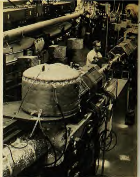
CEA 2-GeV colliding-beam device is now producing peak currents of about 15 mA. Bypass is in front and synchrotron in rear. Technician stands at the interaction region, which is now surrounded by detection apparatus.
