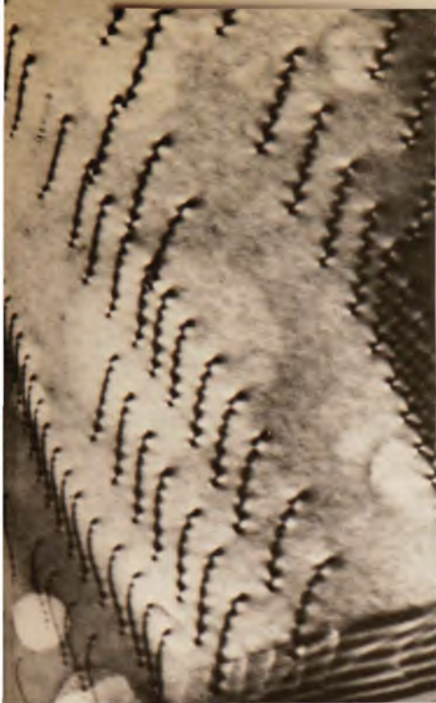
Work hardening in an aluminum alloy. Dislocations are shown piled up against barriers in the crystal. Such pile-ups exert back stress on the dislocation source; so that an increasing amount of shearing stress must be applied to the crystal for the source to operate, resulting in work hardening. Photo provided by Neville Carter of Earth and Space Sciences Dept. of SUNY (Stony Brook) was taken by K. C. Jain, Dept. of Engineering SUNY (Stony Brook).
