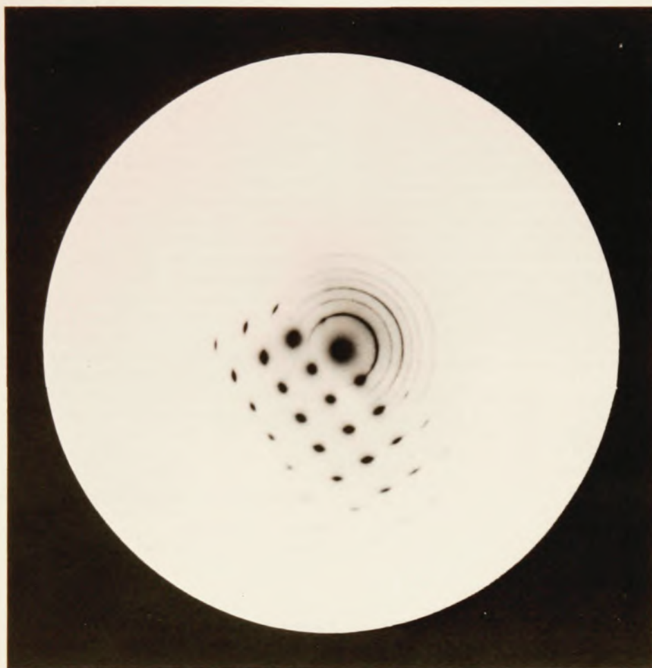
Electron diffraction from a thin film, which is partly polycrystalline and partly a single crystal. The photo, by Sigrid Herd of IBM Corporation is included in Physics from the Ground Up .
