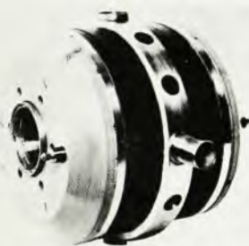
Field 50G, homogeneity to 1 part in 10^9 over 1cm d.i.v. Axial bore 5.2cm - 2 radial apertures of 2.5cm
