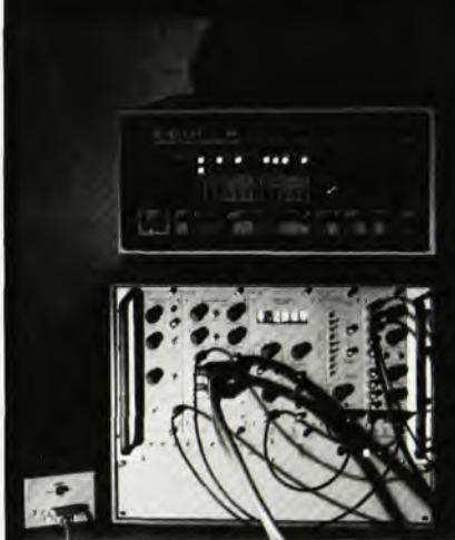
The P.A.R. Model 131 series of modules can keep your instrumented system going day or night. They interface your instruments to a calculator (such as the Wang 700), a mini-computer or a time share computer system. And not only will our 131 series modules acquire and reduce data automatically but they can provide **control** of the instruments generating the data. If the modules listed below can't keep your instruments awake at night, call us—we've got lots more.
