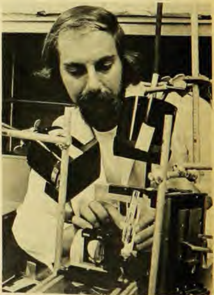
X-ray laser? Light from neodymium-glass laser passes through condensing lens and cylindrical lens (next to hands of John Kepros). Light then strikes copper gel sandwich. At right and rear are x-ray cameras; at left and above are ionization chambers.
