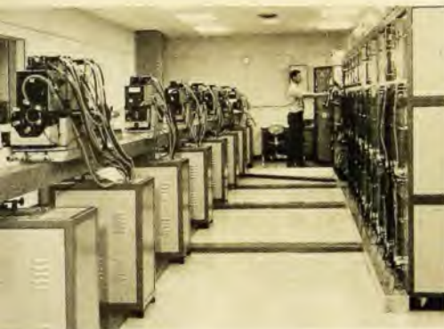
Hadron CGE-640 neodymium-doped glass laser is pulsed at 100 joules in 1 nanosec. Beam strikes target and produces broad-band x-ray source.
