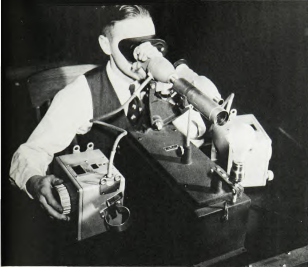
Optical pyrometer. Calibration is carried out with a light source and a standard optical pyrometer. (Photo courtesy of Leeds and Northrup Co).
