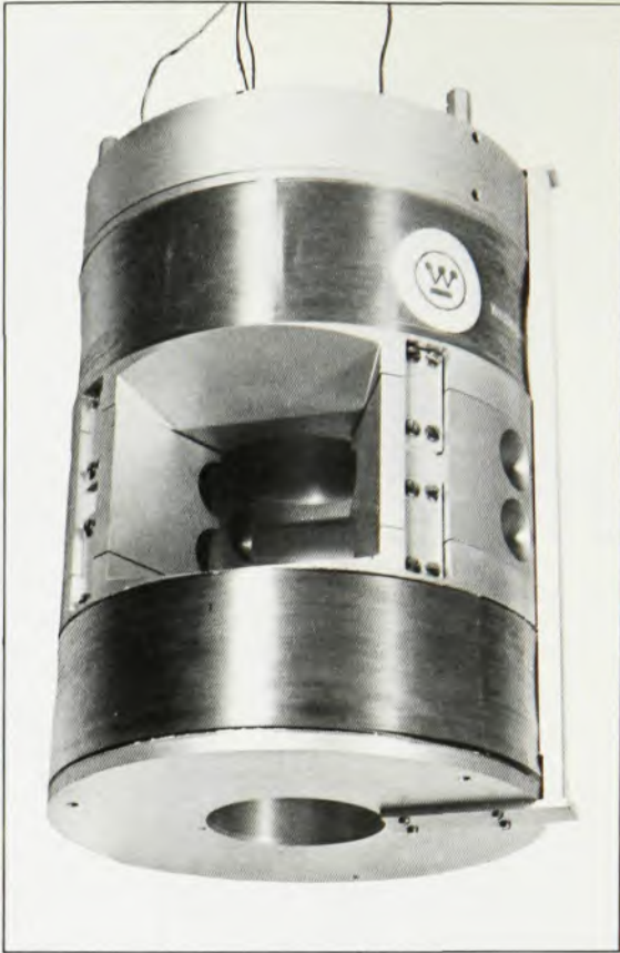
Split coil for neutron diffraction studies, which require access to the magnetic field in both radial and axial directions. (South African Atomic Energy Authority.) Figure 2
