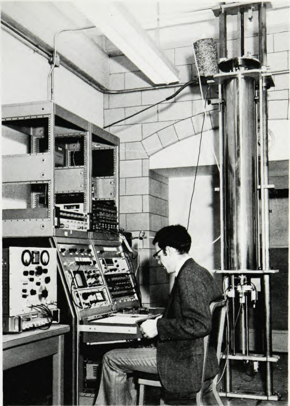
High-uniformity superconducting magnet with which the NMR spectrum of figure 5 was produced. Table 3 shows its long-term drift characteristics. (Carnegie-Mellon University.) Figure 6
