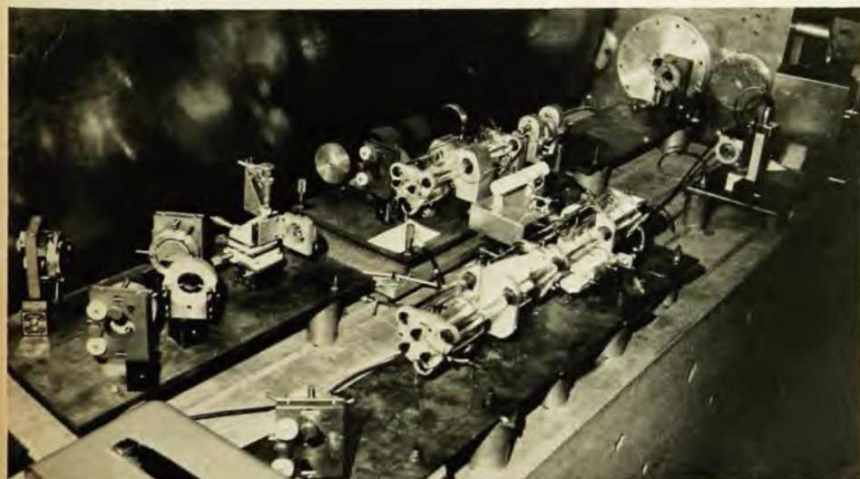
JILA earth-strain gauge in Poorman's Relief Mine near Boulder, Colo. uses a methane-stabilized laser (foreground) as an "absolute" reference. A second laser (center) is mode matched and locked to a 30-meter Fabry-Perot interferometer (right).
