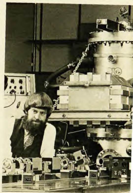
Photofragment spectrometer is used at La Jolla to study dissociative molecular reactions. Beam from laser (on table in front of Kent R. Wilson) enters vacuum chamber (behind Wilson) and interacts with molecular beam. Resulting fragments are analyzed by a quadrupole mass spectrometer that is also within the vacuum chamber.
