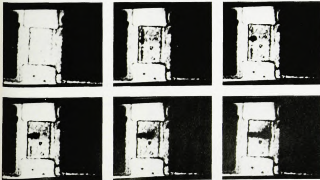
Injection Phenomenon: Stroboscopic photographs of a developing current filament in a silicon-on-sapphire avalanche diode at constant current. From R. A. Sunshine, M. A. Lampert, Appl. Phys. Lett. 18, 468 (1971).
