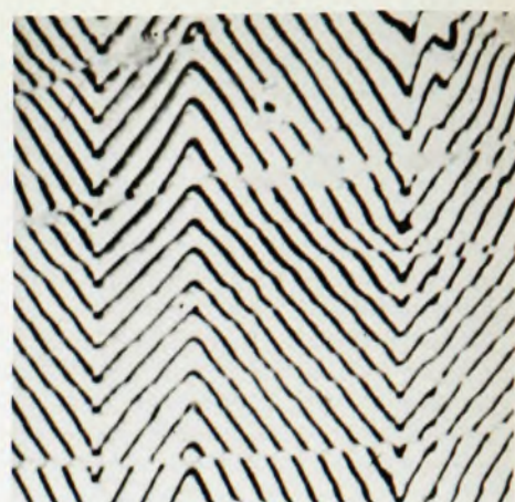
Bismuth single crystal. This interferometric micrograph of a cleavage face shows fairly flat surfaces meeting at an angle; the angle is highly magnified by the interference process and in this example is much less than one degree. (From reference 14.) Figure 11
