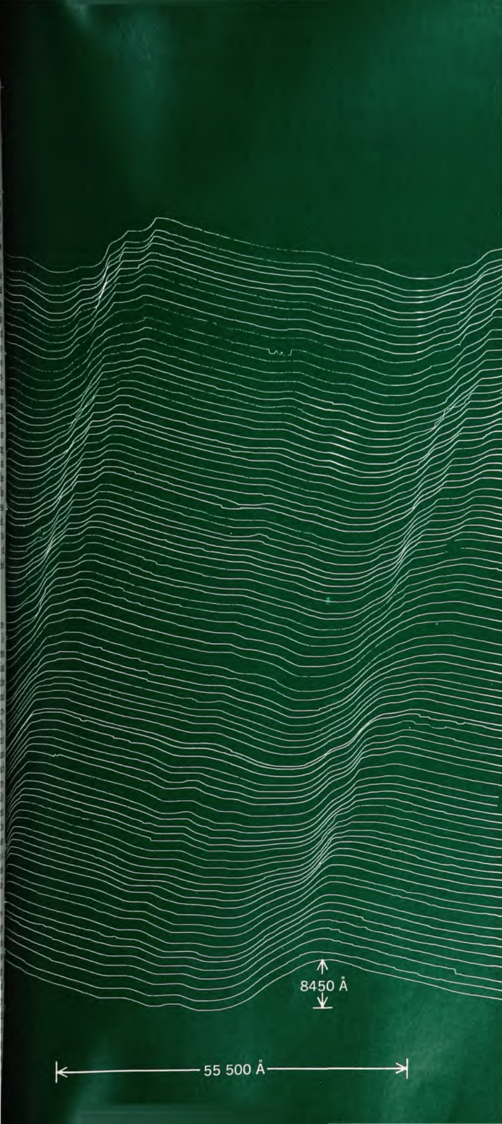
Topographic map of a 180-line-per-mm diffraction-grating replica, obtained with the "topografiner," a noncontacting field-emission probe developed at NBS. Figure 1
