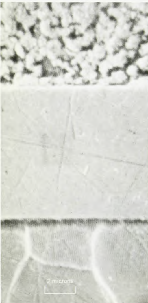
Copper-nickel-steel sandwich , shown in a scanning-electron micrograph. The sandwich was sectioned, highly polished, and lightly etched with nitric acid. The copper surface (above) was roughened by the etch; grain boundaries were exposed on the stainless-steel surface (below), and the nickel (center) retained the fine polishing scratches. (From David Ballard, NBS.) Figure 7
