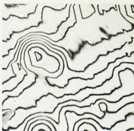
Electropolished nickel single crystal photographed by multiple-beam interferometry. Note the deep etch pits and surface roughening produced by the electropolishing process. (From reference 14.) Figure 10
