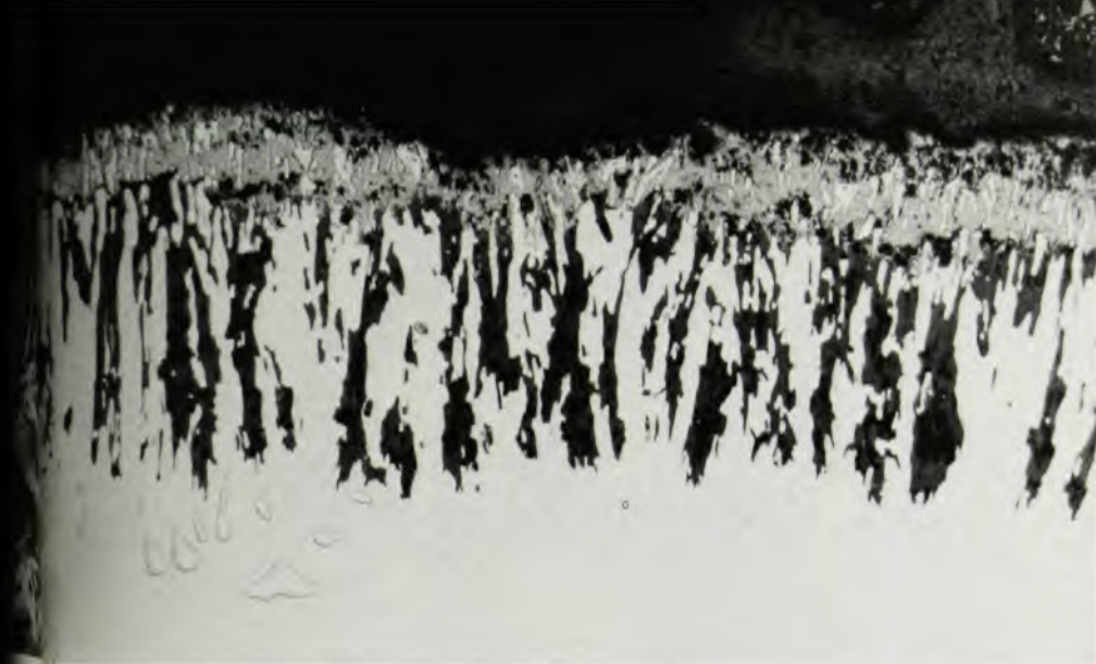
Corrosion in a nickel-tungsten eutectic alloy is shown here in a photomicrograph at about 750 \times magnification. Surface phases are mixed nickel and tungsten oxides. Figure 4
