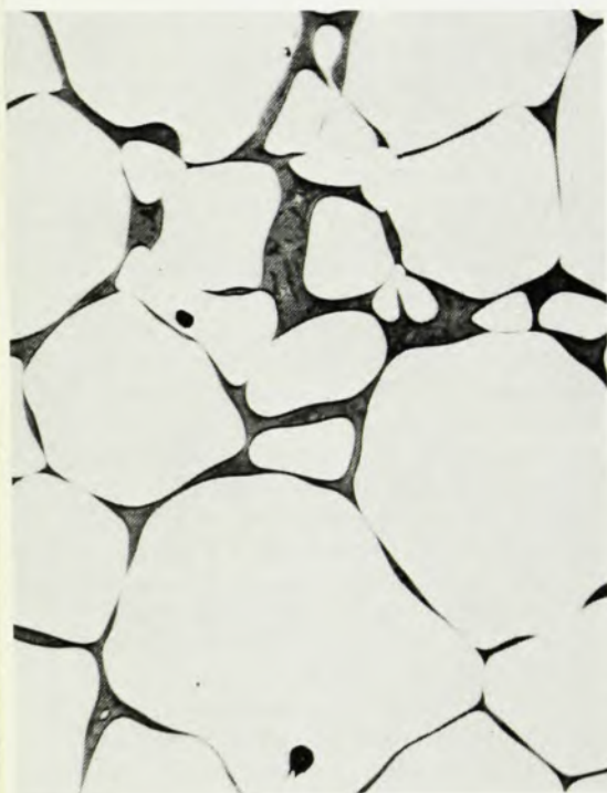
Calcia-stabilized zirconium oxide. Its unusually high conductivity led to a new theory of ionic transport. Figure 6
