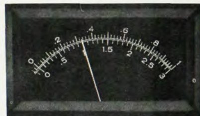
Range 3 millivolts full scale, 10^{12} ohm input resistor. (Equivalent to 10^{-15} amps.)
