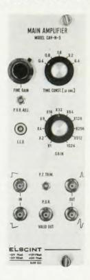
THE ELSCINT MAIN AMPLIFIER MODEL CAV-N-3 HAS A HIGHLY EFFECTIVE PILE UP REJECTOR WHICH GREATLY ENHANCES PERFORMANCE AT HIGH COUNTING RATE, WITH NEGLIGIBLE COUNTING LOSSES.
