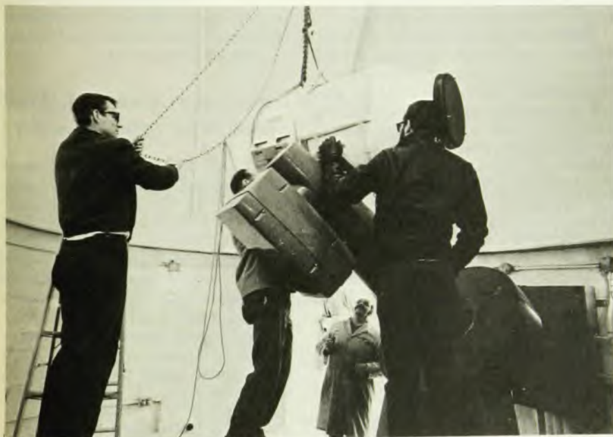
NEW f/2 SCHMIDT TELESCOPE at Goddard Space Flight Center is designed for fixed-focus astronomical observations in the presence of changes in ambient temperature. This feature is desirable in photographing comets that are close to sun and can only be observed for short times at dusk and before dawn. Design employs low-expansion CER-VIT rods to maintain spacing between 23-inch CER-VIT primary mirror and focal region assembly. Telescope will also be used to probe solar wind at remote locations by recording orientations of ionized gas components of comet tails. Photo shows comet camera being lowered onto telescope mount.
