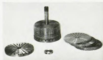
Superconductive Nb 3 Sn tape modules for versatile magnet construction.
