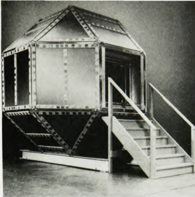
SHIELDED ROOM now operating at MIT has residual magnetic field of 100 nanogauss. It uses three layers of high-permeability alloy and two layers of aluminum. When photo was taken, three sets of double doors had not yet been installed.
