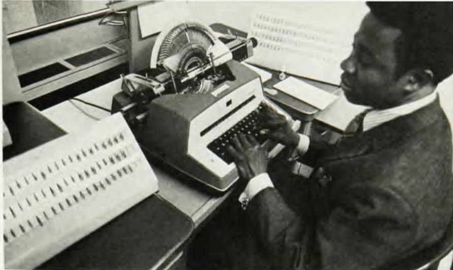
TYPEWRITER COMPOSITION , by which AIP hopes to improve publication speed. The complex typewriter-like machine is operated by Wallace Ross in this photo.
