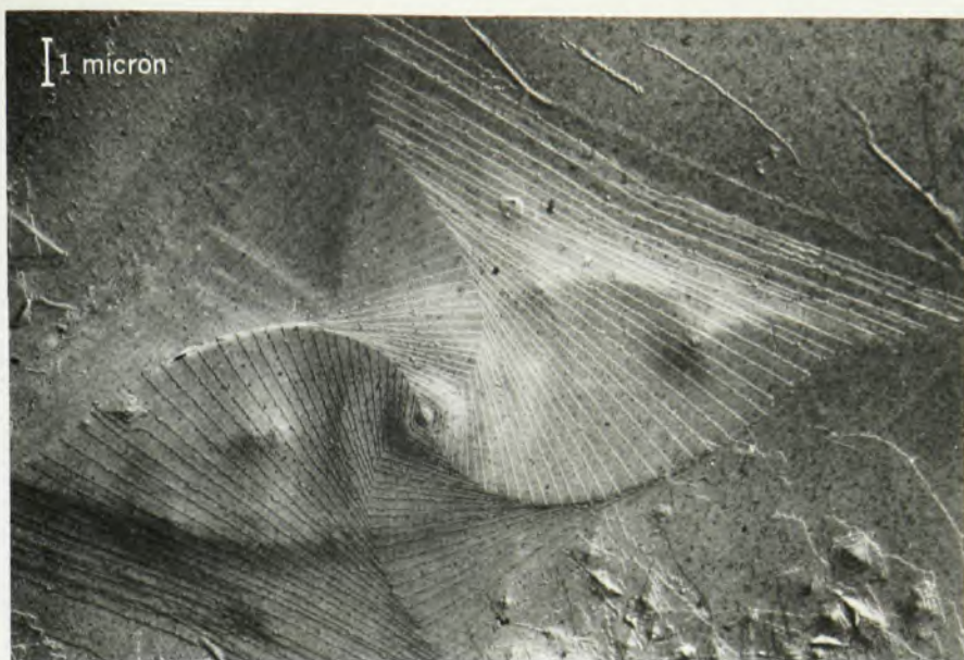
REGULARLY ROTATED TERRACES can be seen in this electron micrograph of a polyethylene crystal replica. From ref. 9. —FIG. 9
