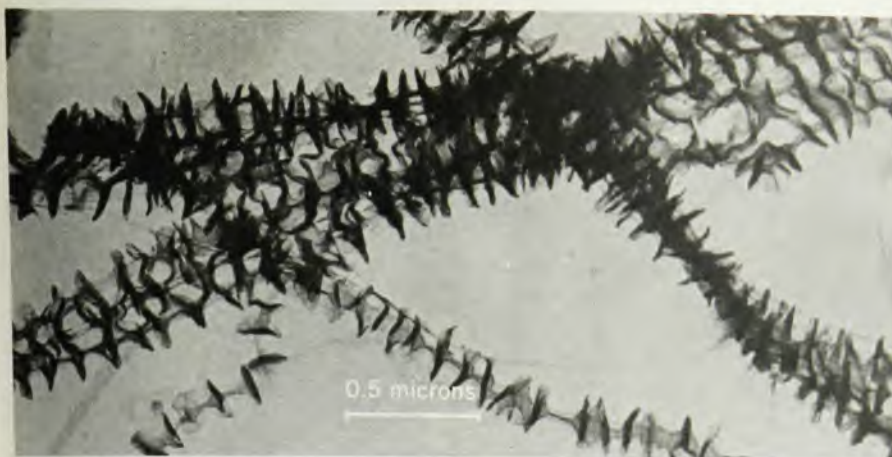
"SHISH-KEBABS" grown in an agitated xylene solution. Electron micrograph shows fibrillar crystals with lamellar overgrowth. From ref. 12. —FIG. 12
