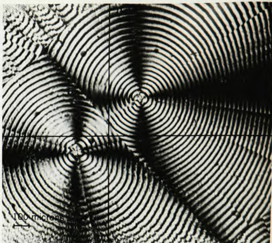
SPHERULITES of poly(trimethylene glutarate) grown between glass surfaces. Photomicrograph with crossed polarizers shows concentric banding associated with helicoidally twisted arrangement of crystals. From ref. 11. —FIG. 11
