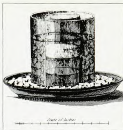
AN EARLY HEAT EXPERIMENT. With this apparatus, Rumford found that an undisturbed vessel of water remains liquid at the bottom when surrounded by a freezing mixture and frozen at the top.
