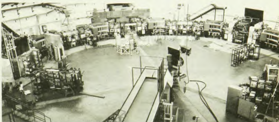
In Adone storage ring at Frascati electrons and positrons collide, each with 1.1 GeV.
