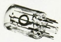
Next we took the Channeltron, put it in a glass tube, added an S-20 photocathode with high red spectral response and a sensitivity of at least 80 microamperes per lumen. Then, we put these high quality parts together with the typical skill that has made Bendix a leader in electronics for decades. We ended up with a Channeltron Photon Counter Tube, which is also the best in its field.
