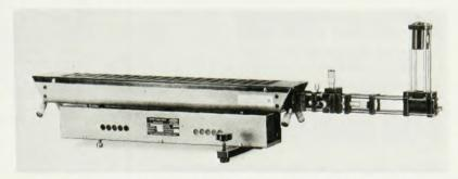
In minutes, a micro optical system containing (among other things) a spatial filter, a beam expander, and a beam steerer has been coupled to the laser to make up a specialized instrument with precise automatic alignment and quickly available microadjustments.
