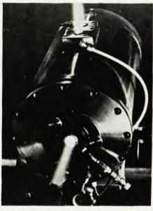
Astro's new MODEL 1000A ULTRA-HIGH TEMPERATURE FURNACE is designed for general lab use with inert, oxidizing or reducing atmospheres, or vacuum—and features a 2.4 inch diameter by 6 inch long hot zone with a heat-up time of 20 minutes to 2700° C.
