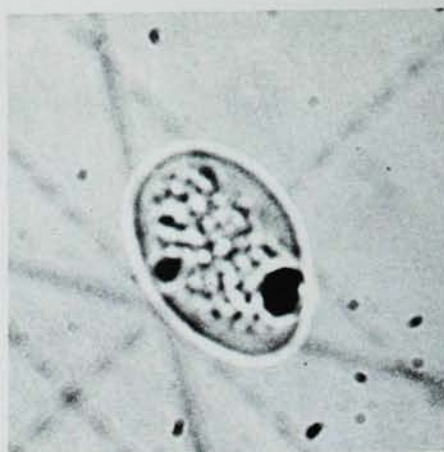
POLYWATER MAGNIFIED 80 times shows birefringence (white areas). Dark spots are voids in the material, which was dropped onto a surface from a capillary. (Lines are from the microscope eyepiece).
