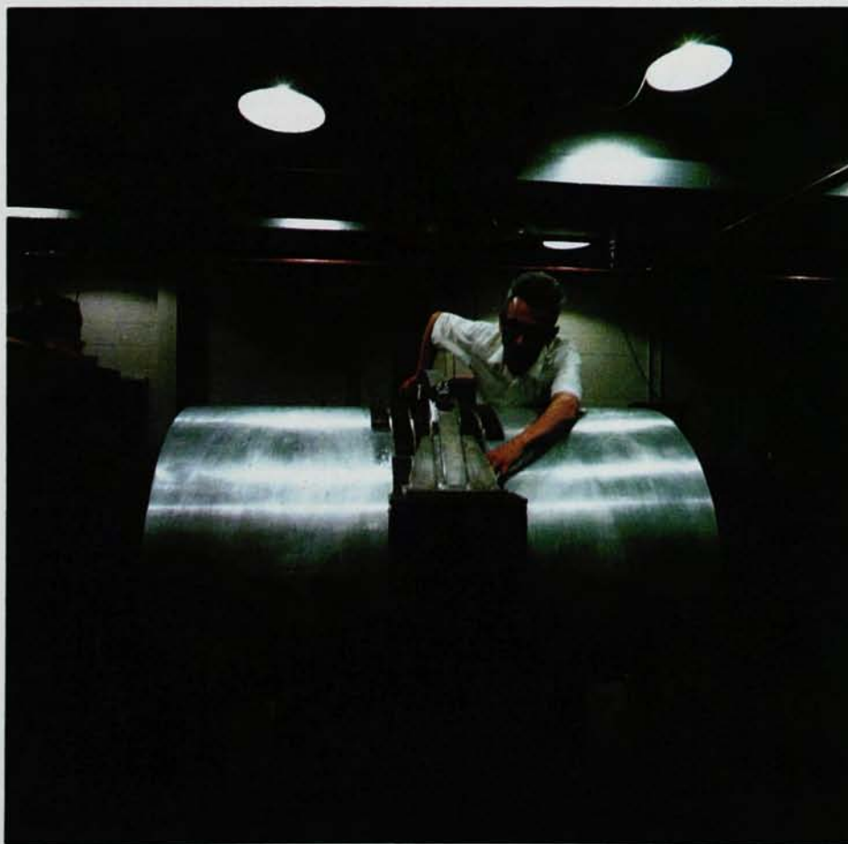
GRAVITATIONAL-WAVE DETECTOR. Joseph Weber of the University of Maryland inspects the suspension of one of the aluminum antennas used to detect waves from extraterrestrial sources. This one is 96 cm in diameter and 153 cm long. It oscillates in response to the Riemann curvature tensor. Weber observed coincidences between detectors in Argonne and Maryland, along a 1000-km baseline.
