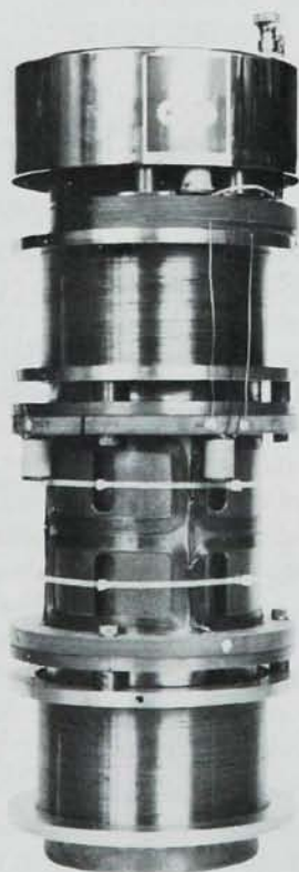
80 Kilogauss N.M.R. Magnet Homogeneity: 3 in 10 7 over 0.9 cm dsv
