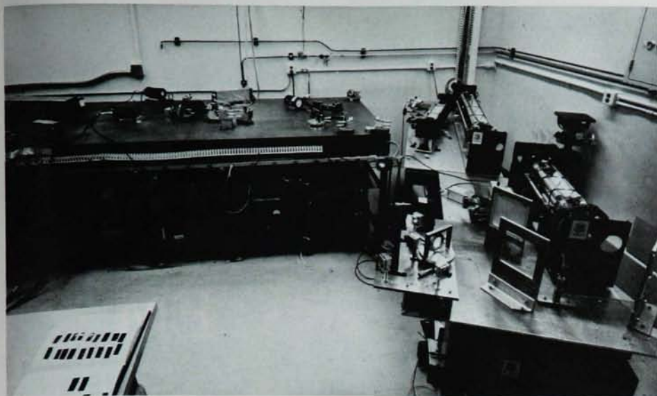
SANDIA LASER has emitted 50 joules in about 2 picosec. Overall gain is 50 000 to 150 000. The mode-locked neodymium-doped glass laser has four amplifier rods. Table at left is 4 meters long; two tables at right are 3 meters long.
