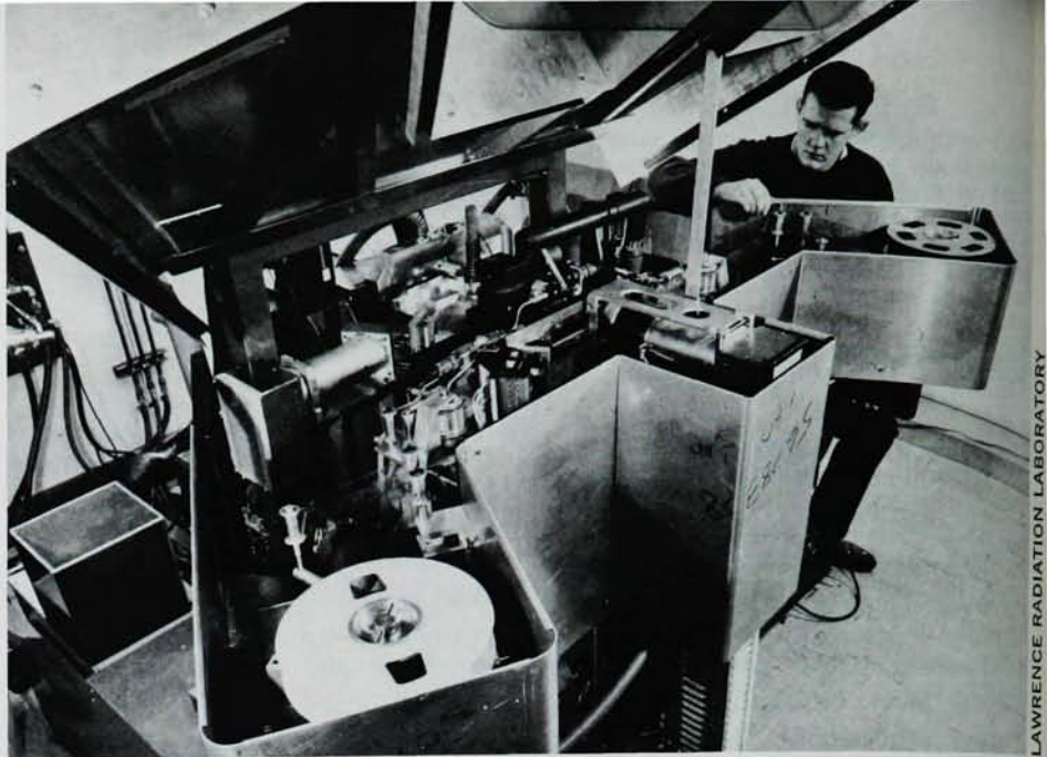
FLYING SPOT DIGITIZER. This automatic film reader measures either spark or bubble-chamber photographs under complete control of an IBM 7090 computer. Film is threaded through the instrument from large spool, lower foreground, through the reading station to the spool, center right. A flying spot generating scanning wheel is at center. The intense moving light spot examines the film along line elements as the film is moved on a measuring engine. The measurement of an entire 72-inch bubble-chamber frame is completed in five seconds.
