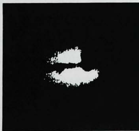
ELECTRON-RING CROSS SECTION was photographed (by the Berkeley group) with its own synchrotron light. Black dot and line are caused by camera grid. Height of photo represents 9 mm.
