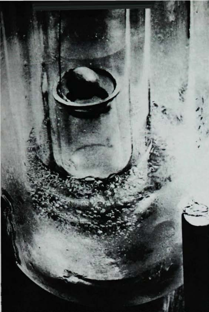
SUPERCONDUCTIVITY. Lead ball cooled below transition temperature is held up by persistent currents.
