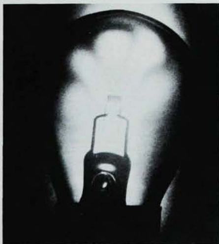
INTERFERENCE FRINGES produced by heated gas inside an automobile dome lamp. The laser hologram that produced the image was exposed first with the lamp unlighted and then, after a four-minute delay, with the lamp lighted.
