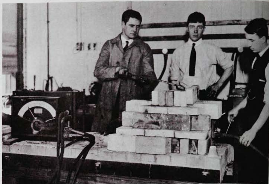
WITH AN ELECTRIC ARC FURNACE producing carborundum from silicon and carbon, MIT students determined conditions for maximal yield and efficiency.
