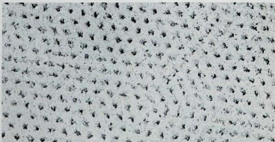
FLUX-LINE LATTICE on the surface of lead with 6.3 atomic per cent indium, at a magnification of 8300. (U. Essman, H. Trauble, Phys. Letters . 24A, 526, 1967.)
