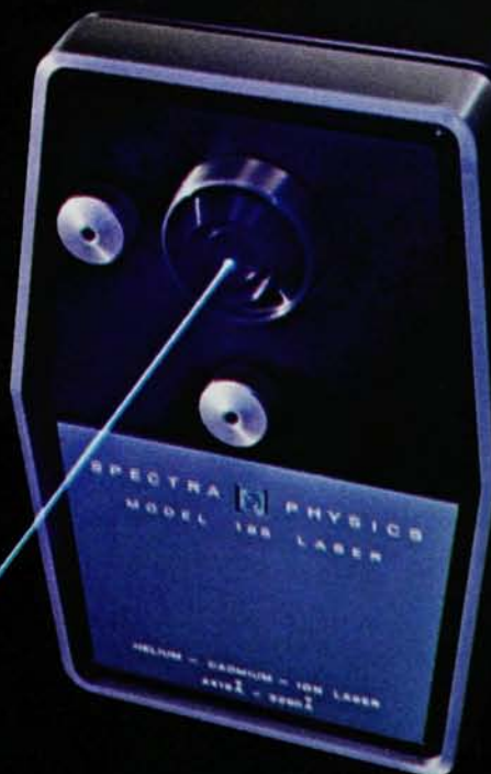
Spectra-Physics Model 185 Helium-Cadmium Laser. Easy to use, reliable, air cooled, it provides 50mW of CW blue @ 4416Å and 5 mW of ultraviolet @ 3250Å.
