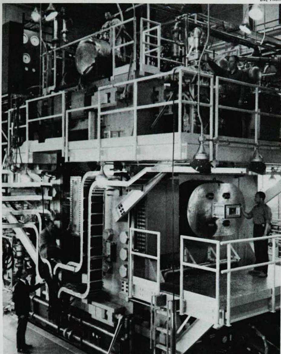
**BUBBLE CHAMBER.** This 80-in. instrument is used with the alternating-gradient synchrotron at Brookhaven National Laboratory. The large aperture at lower right is for the source of illumination; around it are four smaller apertures for cameras. The hydraulic ram below the chamber moves the entire assembly along a rail track.
