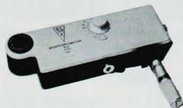
MONOCHROMATOR , miniature quartz prism type, F/7.6 Range 190-1500 mμ. Slits are adjustable in unison.
