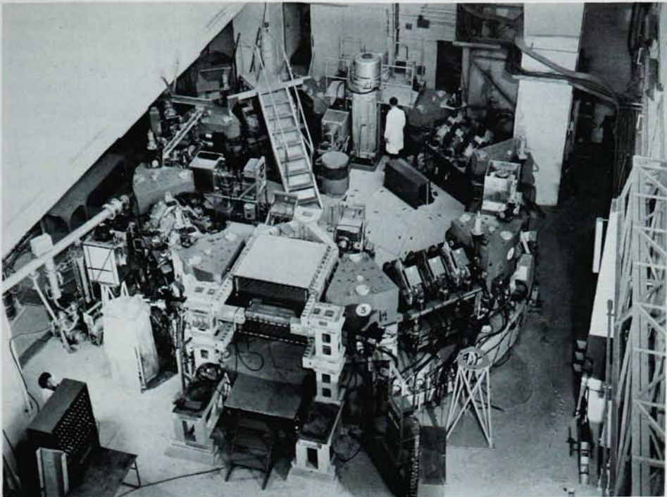
STORAGE RING for colliding beams of electrons and positrons at Orsay. This ring stores beams of over 500-MeV energy each. Annihilation of electrons and positrons with pion production measures the pion form factor. —FIG. 2
