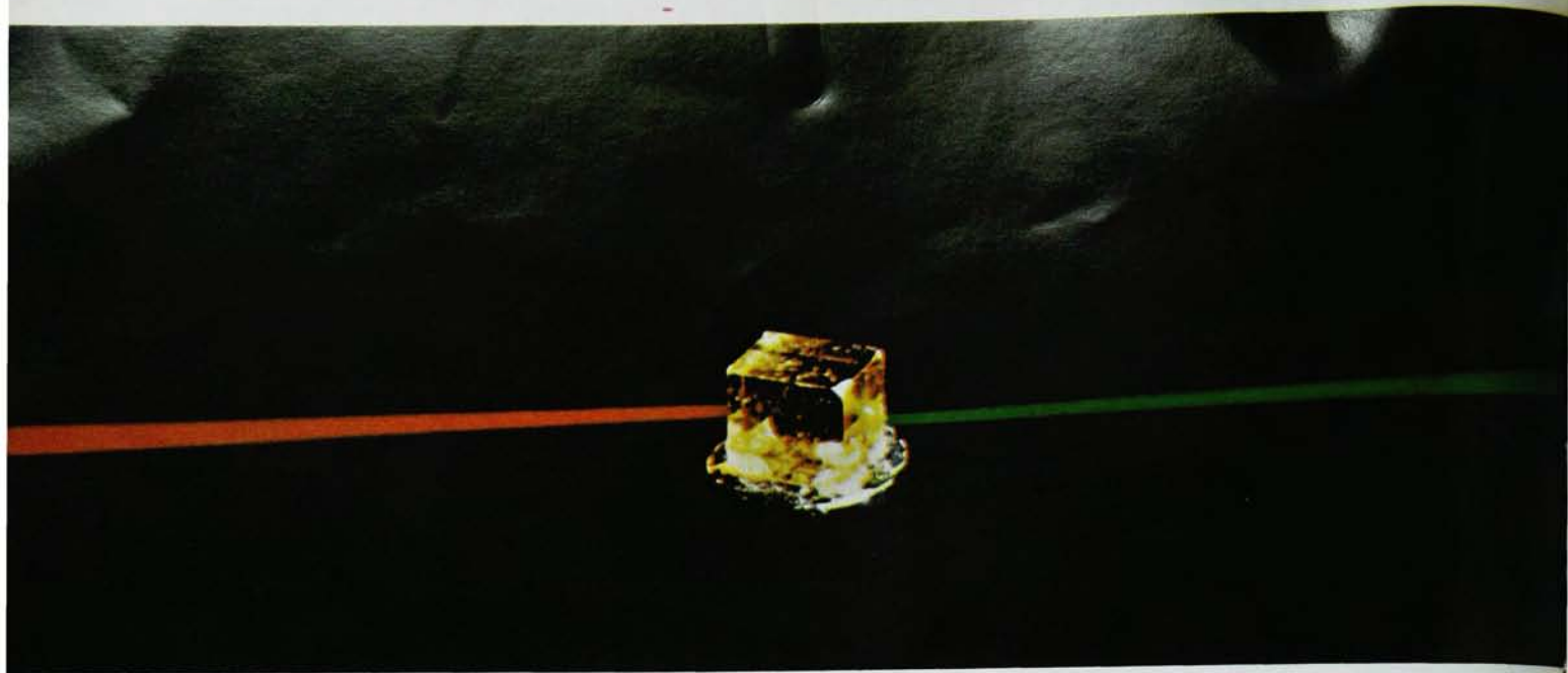
RED-TO-GREEN CONVERSION (above). Infrared laser light (1.06 microns) changes to green second-harmonic light (0.53 micron) in a crystal of barium sodium niobate. This photograph was made with the aid of a card treated with infrared-sensitive phosphor. In work by J. E. Geusic, H. J. Levinstein, S. Singh, R. G. Smith and L. G. Van Uitert at Bell Telephone Laboratories a similar crystal mounted in a 1-watt 1.06-micron continuous-wave laser has produced 1 watt of continuous 0.53-micron light.
