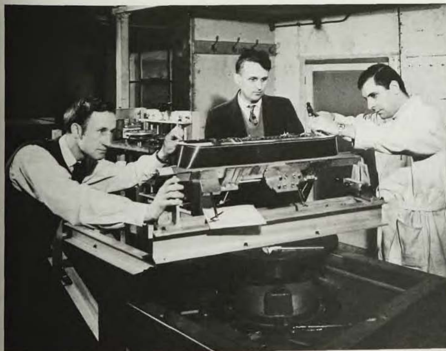
MARTIN WOOD, HEAD OF OXFORD INSTRUMENT CO., directs manufacture of superconductive quadrupole magnet for CERN, the first such unit built commercially.
