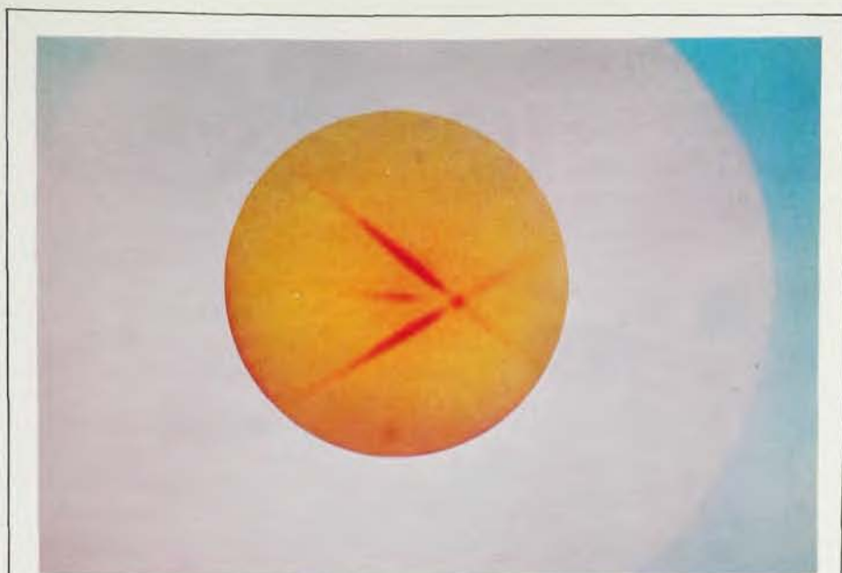
PROTON CHANNELING IN SILICON. R. Stuart Nelson (AERE Harwell) used ordinary color film (Agfa CN-17) as an energy analyzer to obtain this picture of 1.5-MeV protons that have passed through a silicon single crystal 30 microns thick. Randomly scattered protons lose some energy in the crystal and are stopped in the yellow emulsion of the film; protons that traverse the crystal along preferred crystal-plane directions known as "channels" lose less energy and can penetrate to the next emulsion layer to yield a red image. Total film thickness is 20–22 microns. Asymmetry in the pattern is caused by a 3-deg tilt of the film plane with respect to the 100 plane of the crystal. The method is reported in Journal of Materials Science 2, 171 (1967).
