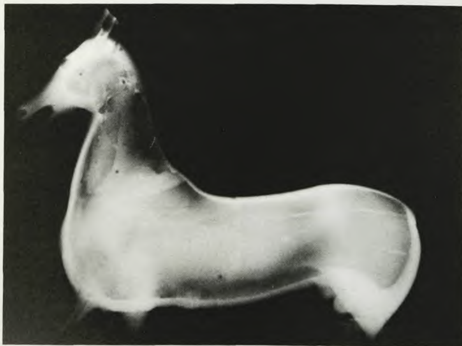
GAMMA RAY SHADOWGRAPH of the Bronze Horse in the Metropolitan Museum of Art, made with iridium 192. Inner sand core and iron wires are thought to indicate modern construction. (Photo: Metropolitan Museum of Art 1967.)
