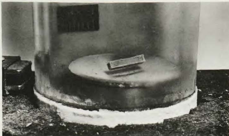
SMALL BAR MAGNET floating on its own magnetic field. The frosted lead dish beneath it has been made superconducting by immersion in liquid helium at 4 K; the field lines excluded from the superconducting material levitate the magnet. This photograph was made at the Lewis Research Center of NASA.
