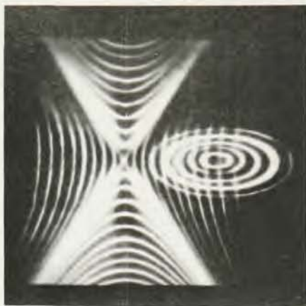
3D IMAGE depicted in this integral photograph is of a computer-generated surface showing contours. The actual image had a depth of 15 cm. —FIG. 9
