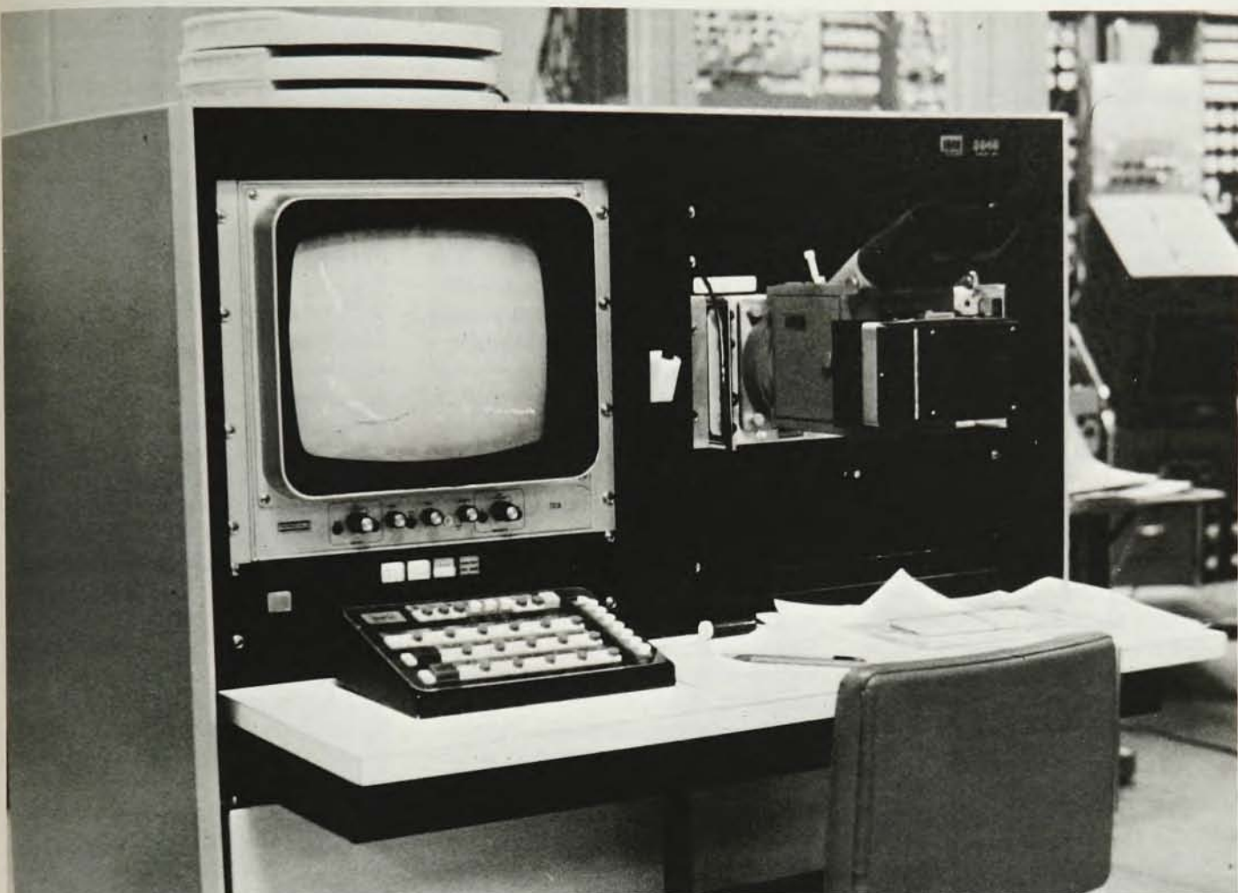
COMMUNICATIONS TERMINAL showing the display CRT, light pen and function keyboard. The oscilloscope at right is connected with large CRT and is used for photographic purposes. —FIG. 2
